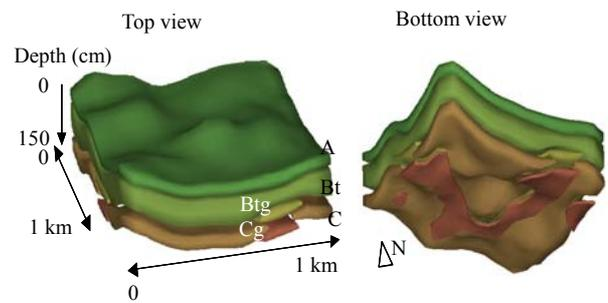
**Fig.4 3D stratigraphic model showing the spatial distribution of soil horizons. Soils on elevated areas: Plano, Ringwood and Saybrook Series (fine-silty, mixed, mesic Typic Argiudolls); soils in depressions: Joy and Ossian Series (fine-silty, mixed, mesic Aquic Hapludolls and Typic Haplaquolls, respectively)**
